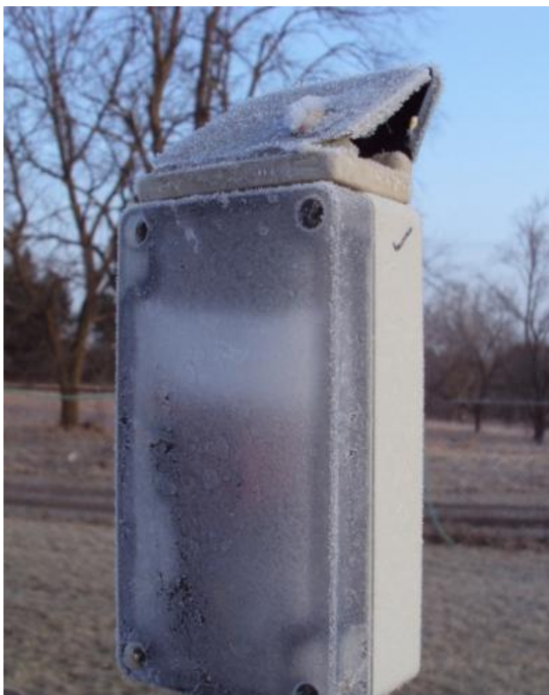
Figure 4. Sensor nodes based on solar panels and rechargeable batteries typically have problems associated with sub-zero temperatures.
